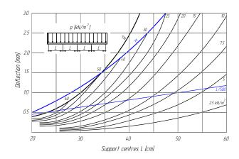
Flexural stiffness El=3.1 kNm<sup>2</sup>/m (15% timber moisture content)
