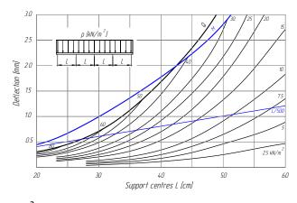
Flexural stiffness El=4.7 kNm<sup>2</sup>/m (15% timber moisture content)
