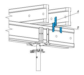
To prevent the secondary beam stipping on their sides while the panels are being laid on them, rafter plates can be used.
