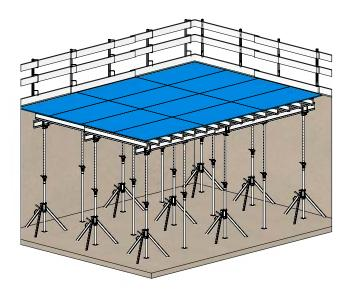
Where necessary (e.g. edge zones), secure the panels with nails. Recommended nail lengths for the plywood thickness 18-21 mm - approx. 50 mm
