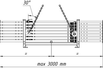
Only lift the boxes when their sidewalls are closed. Do not exceed the permitted load-bearing capacity.
