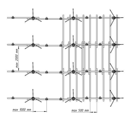
The primary beams should be oriented at right angles to the direction of an uneven length/width of room (5 m, 7 m, 9 m, etc.). This makes more efficient use of the potential of the system.
