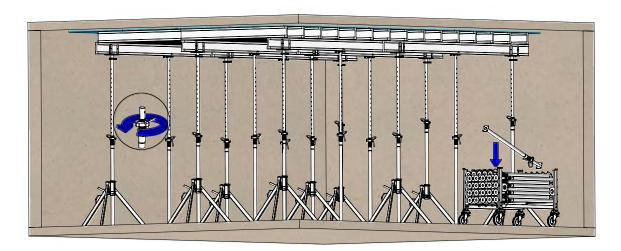
After the intermediate props have been removed, there usually remain only props spaced 2.0 m apart in the direction of the secondary beams and 3.0 m apart in the direction of the primary beams. This leaves enough space to maneuver wheel-around scaffolds and stacking pallets without difficulty.
