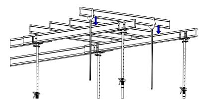
Measure up the positions of the secondary beams.
