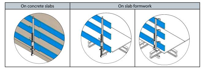
Only attach the Guide rail clamp to formwork beams if these cannot tip over. Never mount guard-rail boards in the longitudinal direction of the formwork beams. It is forbidden to fasten the clamp to the formwork sheeting only.
