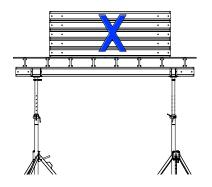
It is not permitted to set down any loads on the floor-slab formwork (e.g. beams, formwork sheets, reinforcement steel) until the intermediate props have been set up.
