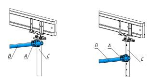
Before fitting the bracing, make sure that the holes in the floor prop or lowering head are correctly aligned.
