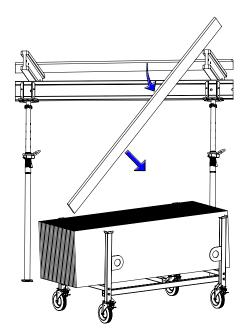
Remove the remaining secondary beams and the primary beams, and put them in the stacking pallet.
