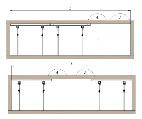
L ... Effective floor-slab spans of 7.50 m and over
