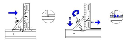
The diagonal bracing of the beam forming support ensures that the joint between the plywod sheets is automatically pressed together tightly when the beam forming support is clamped.
