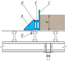
d = slab thickness max. 30 cm
